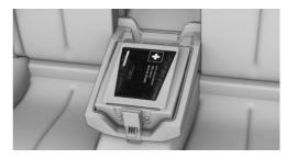
When replacing the insert, place both pins into the rail at the bottom and press the insert back in place until a 'click' is heard. Ensure that the rear seat backrest upholstery is not damaged.
