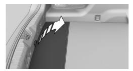
The tow fitting is located in the onboard vehicle tool kit under the cargo floor panel.
