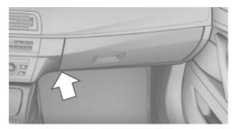
Socket is located below the glove compartment.
