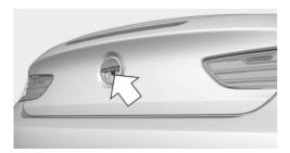
The camera lens is located under the BMW emblem of the tail gate. The image quality may be impaired by dirt. The camera calibrates itself regularly after the system has been switched off. This is why the emblem on the tailgate remains open after the system has been deactivated and while driving. The emblem closes automatically as soon as calibration is complete.
