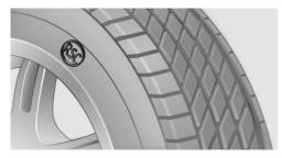
RSC label on the tire sidewall.
