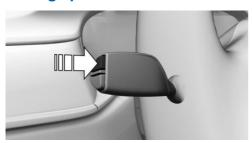
Press and hold button on signal lever.
