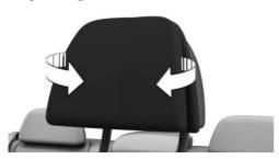
Fold the side extensions on the head restraint forward for increased lateral support in the resting position.
