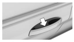
Grasp the handle of a vehicle door completely. This corresponds with pressing the button ? on the remote control.
