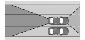
Four radar sensors in the bumpers monitor the area next to the vehicle in the speed range from approx. 45 mph/70 km/h to approx. 130 mph/210 km/h.
