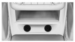
The center console contains one or two sockets. Pull off the respective cover.
