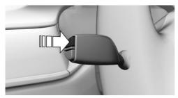
Press and hold button on signal lever.
