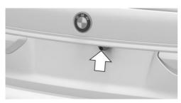
The camera lens is located in the handle of the tailgate.
