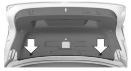
3. Press against the interior trim, arrows, so that the four holding pins engage in the tailgate.
