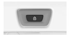
With the driver's door shut, press button on the inside of the tailgate.
