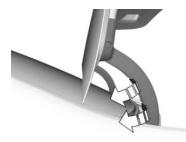
2. On the expanding rivet, carefully pry out the inside pin by a small distance using a screwdriver. Then carefully pry out the expanding rivet all the way using the screwdriver.
