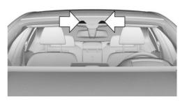
The camera is installed near the interior mirror. Keep the windshield in front of the interior mirror
