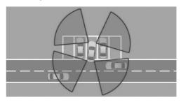
Two radar sensors in the rear bumper monitor the area behind the vehicle.
