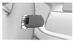
Adjusting the rain sensor sensitivity: Turn the thumbwheel on the wiper lever.
