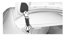
Fasten the hinge cover using the expanding rivet, arrow 1, and press onto the hinge cover so that the holding pin engages in the tailgate, arrow 2.
