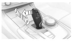
Press the selector lever to the left out of selector lever position D, arrow 1. Next, push the selector lever forward or pull it backward, arrow 2.
