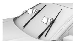
3. Press button, arrow 1, and pull out the wiper blade, arrow 2.
