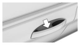
Grasp the handle of a vehicle door completely. This corresponds with pressing the button of on the remote control.
