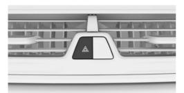
The button is located in the center console. The red light in the button flashes when the hazard warning flashers are activated.
