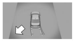
The respective boundary area in the PDC view flashes red, if vehicles are detected by the sensors.
