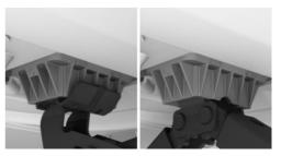
Extend the vehicle jack by turning the crank or lever clockwise.
