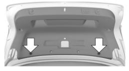
Press against the interior trim, arrows, so that the four holding pins engage in the tailgate.
