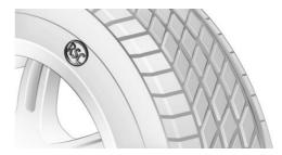
RSC label on the tire sidewall.
