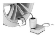
With the compressor switched off, insert the plug into the power socket inside the vehicle.
