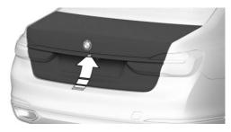
Without Comfort Access: unlock vehicle. With Comfort Access: unlock the vehicle or have the remote control with you. Press button on the exterior of the tailgate.
