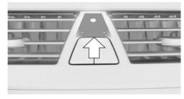
The NFC antenna is in the instrument panel above the hazard warning flashers button.
