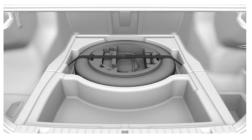
The emergency wheel and the tools are located in the cargo area under the cargo floor panel.
