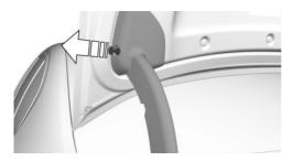
Carefully lift off the hinge cover from the hinge arm, arrow 1, until the holding pin, arrow 2, behind the trim panel is released.
