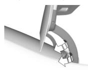
On the expanding rivet, carefully pry out the inside pin by a small distance using a screwdriver. Then carefully pry out the expanding rivet all the way using the screwdriver.
