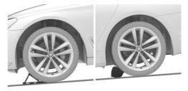
If you need to change a wheel on a slight downhill gradient, place chocks and other suitable objects, for example a rock, under the wheels of both the front and rear axles against the rolling direction.
