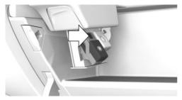
6. Insert the fragrance cartridge without pressure into the cartridge holder. The cartridge snaps lightly into place.
