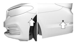
With the four side ultrasound sensors, arrows, and the ultrasound sensors of the PDC in the bumpers, the parking spaces are measured and the distances to obstacles determined.
