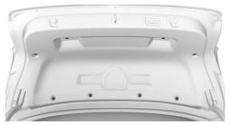
2. Reach into the handle recess on one side and carefully pull the interior trim downward, arrow 1, to the point where the two
