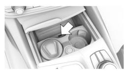
A USB interface is located in the center console.
